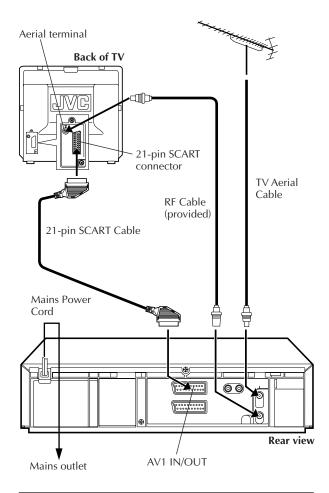
Make AV connection if your TV has a 21-pin AV input connector (SCART) in order to reduce the possibility of interference. And if you are using a stereo TV, you will need this cable in order to enjoy stereo playback of videotapes.
